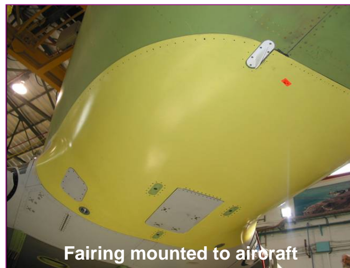
ROHACELL foam core plus stitched-on CF-fabric
