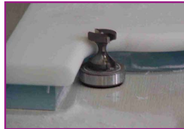
High speed routing
