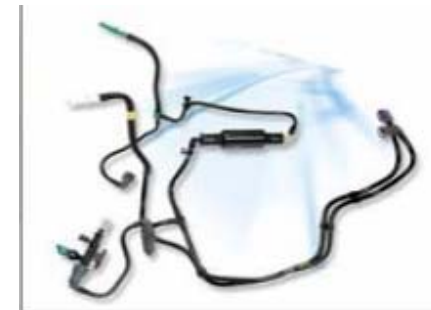
Fuel lines and tubing
