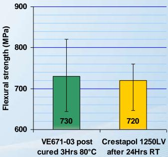
410gsm NCF T700SC fibres 12K tow 50C size [0/90/90/0]s ILSS tests to ISO 14130, Flexural tests to ISO 14125
