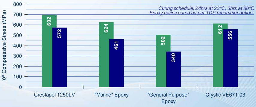
Original strength = tested dry at 23°C ambient
