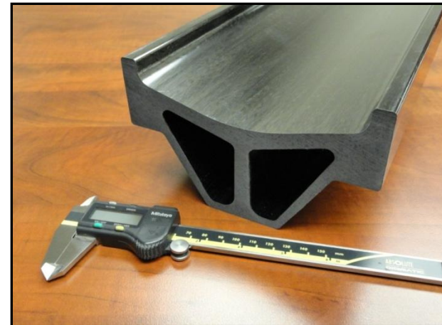
Machine component converted from aluminum to CFRP- weight reduction, increased stiffness 1300 ends of 48k Carbon (max wall thickness 38mm)
