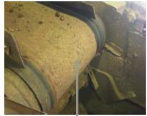
Sediment is NOT destroying belt, through penetrating (since no aging as rubber)
