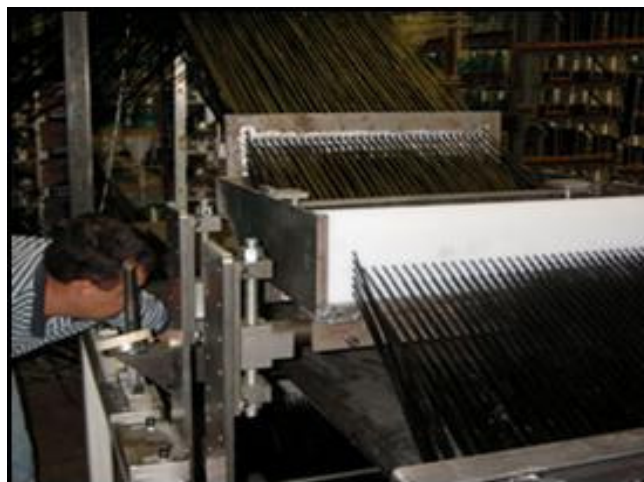
Fiber / Fabric Placement
