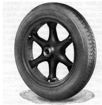
(left) wooden wheel from the early 20 th century and (right) the Georg Fischer Simplex wheel made of cast steel of 1927.
