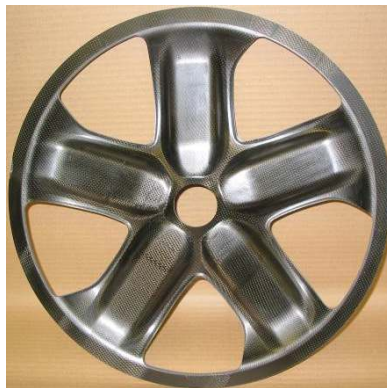
Wheel centre made of carbon fibre reinforced thermoplastics.
